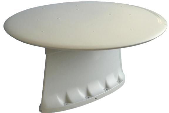
The 19-4001 is a combined broadband VHF/UHF communications and UHF satellite communications antenna. It covers the frequency bands 30-88 MHz and 108-174 MHz for communications, 225-400 MHz for Line-of-Sight (LOS) and Beyond Line-of-Sight (BLOS) satellite communications, and 400-512 MHz for Special UHF requirements.
